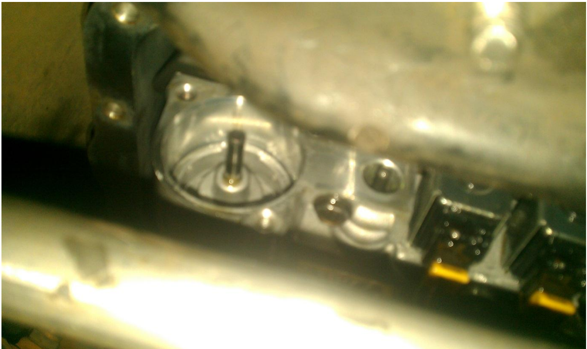
Cover Removed and Springs Removed
