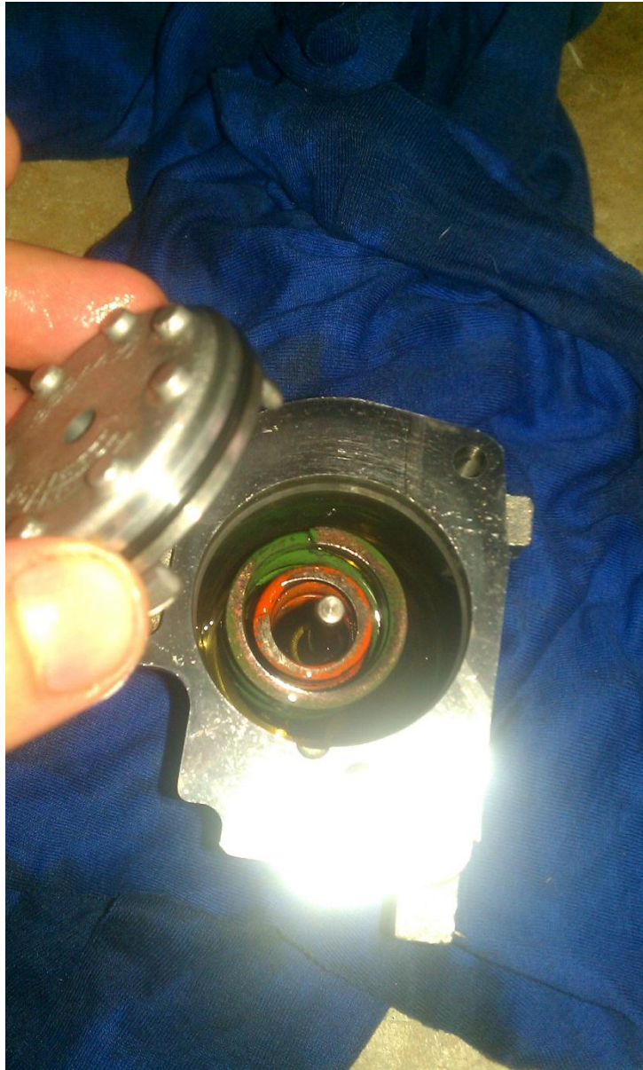
Piston removed here are the springs
