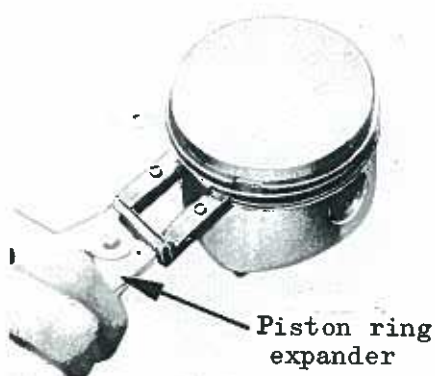
Fig. 4-22 Dismantling 38
